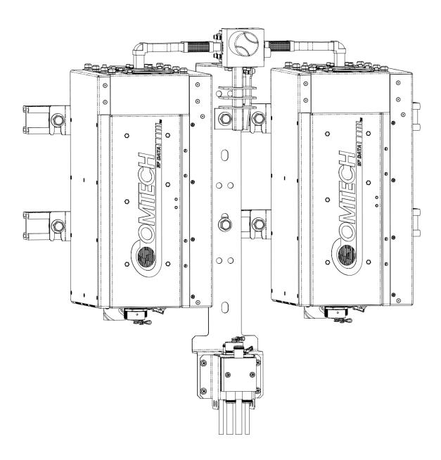
Figure B-15. KT-0021435 LGaN 100 W 1:1 Redundant Ku Switch and Mounting Kit – Assembled Isometric View
