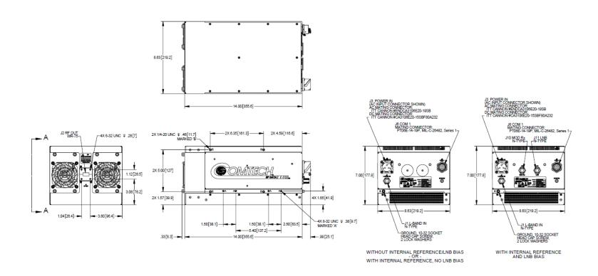
Figure 1-5. LGaN 100 W Ku-Band Dimensional Envelope (1 of 2)
