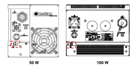
Figure 2-5. LGaN Ground Connector Locations
