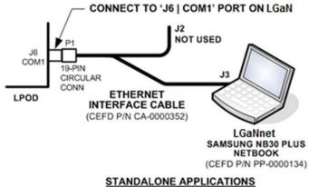
Figure 3-2. Standalone or Redundant Ethernet Connection
