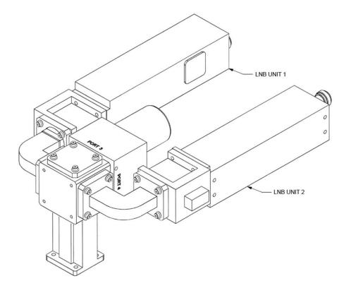
Figure B-9. PL/7596-1 LGaN Ku-Band Rx Switch Kit – Assembled Isometric View
