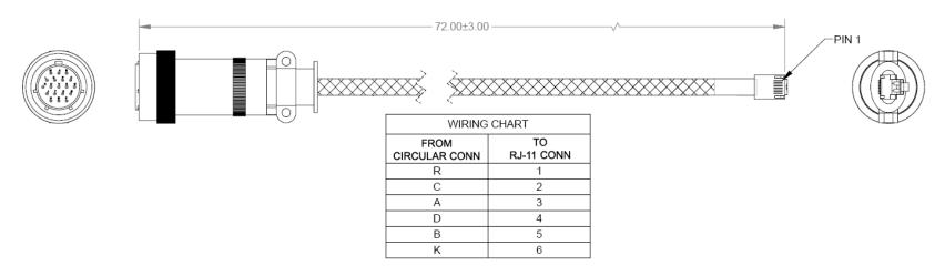
Figure A-1. Serial Interface Cable (CEFD P/N CA-0020526, part of KT-0020518)
