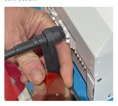
3. Verify the tape covers all of the connector and makes contact with the unit.
