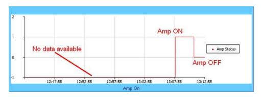
This graph displays the state of the RF amplifier (On/Off). As per this example:
