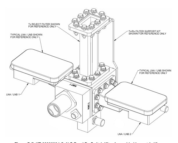
Figure B-7. KT-0000098 LGaN C-Band Rx Switch Kit – Assembled Isometric View
