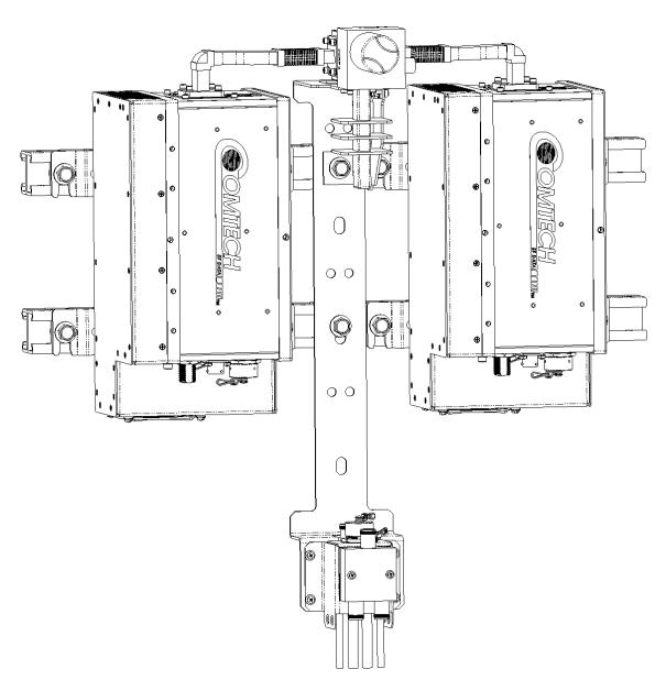
Figure B-13. KT-0021223 LGaN 50 W 1:1 Redundant Ku Switch and Mounting Kit – Assembled Isometric View
